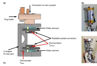
"Huginn: A Peltier-based sub-cryostat for neutron scattering",
